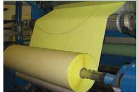
Yellow, dimpled PVC liner on silicone adhesive coating
