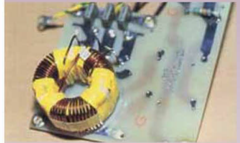
Coil outer wrap taping
