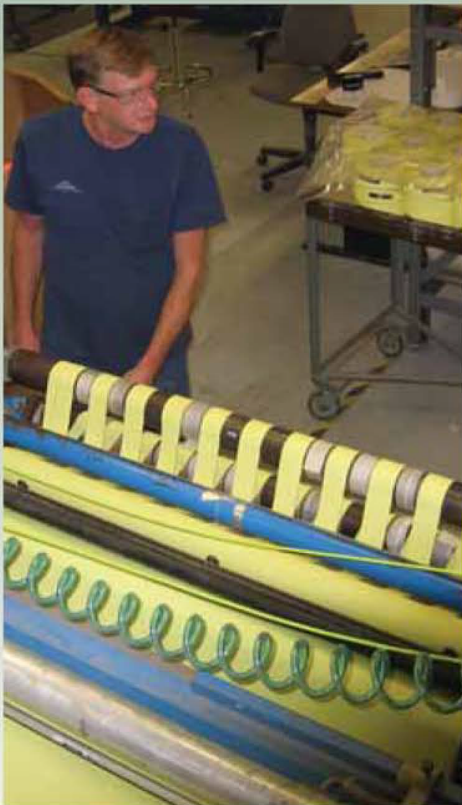
Tape conversion operator on crush-cut, rewind slitter
