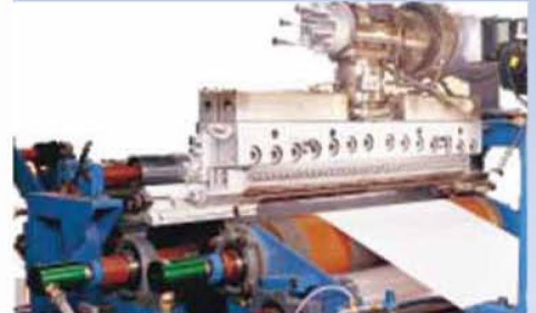
Orange overcoat masking tape on chill roll
