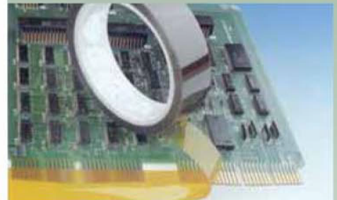
Finger masking with polyimide tape
