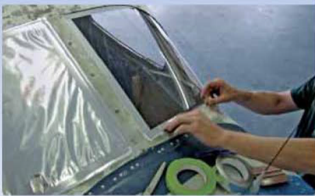
Plane paint masking
