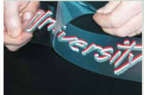
Siliconized PET film liner for college car window graphic
