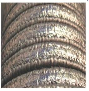
(<u>For best performance</u>: install an SATB, NEBCO Style 1900, or other suitable material at the bottom of the box.)
