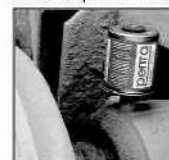
perma Classic providing bearing lubrication and a positive purge of grease to prevent contaminants.
